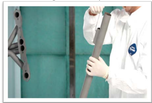
Racking Exhaust Pipes
